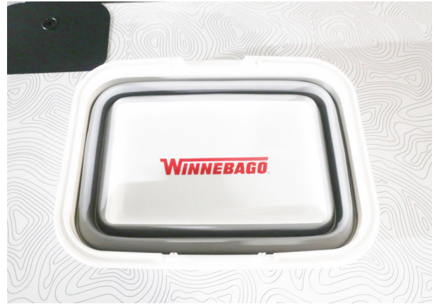
Portable sink shown in the folded up position. Hold on to the sides and push in on the center to unfold the sink. -Typical View
