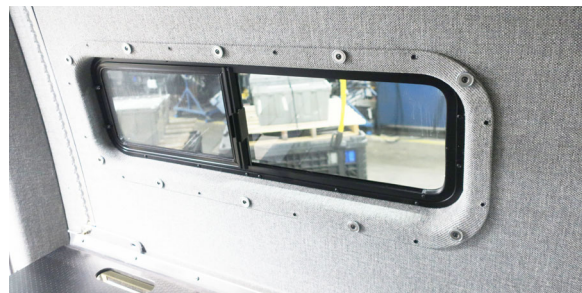
Horizontal Slider Window -Typical View
