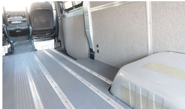
The tracks run throughout the coach, enabling the chair to be placed in many locations. - Typical View
