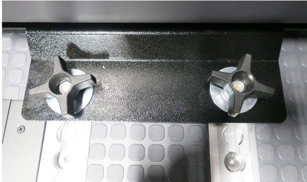
Front track pins- turn counter-clockwise to loosen and clockwise to tighten. -Typical View
