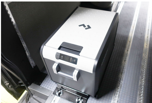
Refrigerator shown mounted on the track system. -Typical View
