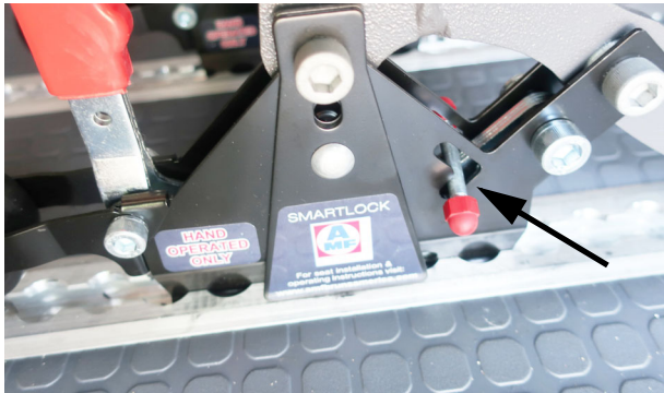
Lift the safety bolt up into the upper position. - Typical View
